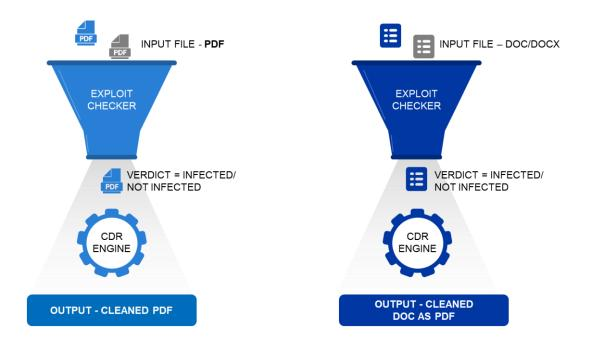
To summarize, when a customer subscribes to CDR API, any attachment that comes from external source in the form of PDF/DOC/DOCX file, the exploit checker processes the input file (PDF/DOC/DOCX) through the CDR engine and shares a cleaned file (PDF/DOC/DOCX) as an output.
